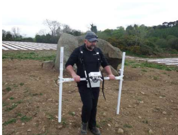
Bartington Grad 601-single axis dual sensor gradiometer.
