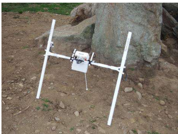
Bartington Grad 601-single axis dual sensor gradiometer.
